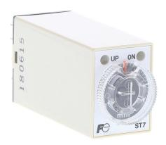
Fuji Electric on-delay relay timer, 4 to 60 minutes selectable timing range, 100-120 VAC operating voltage, 3A contact rating, (1) DPDT timed relay output(s), socket mount, 8-pin. Requires Fuji Electric TP88X2 timer socket.
