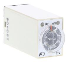
Fuji Electric on-delay relay timer, 0.4 to 5 seconds selectable timing range, 100-120 VAC operating voltage, 3A contact rating, (1) DPDT timed relay output(s), socket mount, 8-pin. Requires Fuji Electric TP88X2 timer socket.
