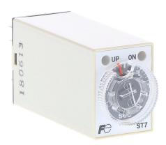
Fuji Electric on-delay relay timer, 2 to 30 seconds selectable timing range, 100-120 VAC operating voltage, 3A contact rating, (1) DPDT timed relay output(s), socket mount, 8-pin. Requires Fuji Electric TP88X2 timer socket.
