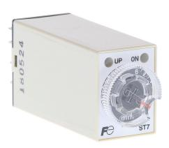
Fuji Electric on-delay relay timer, 1 to 10 minutes selectable timing range, 100-120 VAC operating voltage, 3A contact rating, (1) DPDT timed relay output(s), socket mount, 8-pin. Requires Fuji Electric TP88X2 timer socket.
