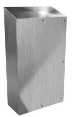
Hammond Eclipse series enclosure, slope top, NEMA 3R/4/4X/12/13, 60 x 36 x 16in (HxWxD), wall mount, 304 stainless steel, #4 brush finish, single-door, 1/4-turn semi-flush 316 stainless steel latch.
