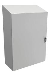
Hammond Eclipse series enclosure, slope top, NEMA 3R/4/12, 48 x 36 x 16in (HxWxD), wall mount, carbon steel, RAL 7035 light gray, powder coat finish, single-door, 3-point keylocking handle.
