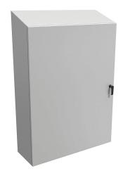
Hammond Eclipse series enclosure, slope top, NEMA 3R/4/12, 48 x 36 x 12in (HxWxD), wall mount, carbon steel, RAL 7035 light gray, powder coat finish, single-door, 3-point keylocking handle.
