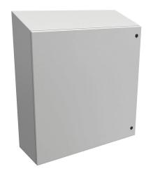
Hammond Eclipse series enclosure, slope top, NEMA 3R/4/12,  $36 \times 36 \times 12$  in (HxWxD), wall mount, carbon steel, RAL 7035 light gray, powder coat finish, single-door, 1/4-turn semi-flush latch.
