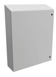
Hammond Eclipse series enclosure, slope top, NEMA 3R/4/12,  $36 \times 30 \times 8$  in (HxWxD), wall mount, carbon steel, RAL 7035 light gray, powder coat finish, single-door, 1/4-turn semi-flush latch.
