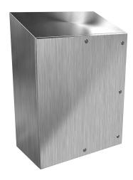
Hammond Eclipse series enclosure, slope top, NEMA 3R/4/4X/12/13,  $36 \times 30 \times 16$  in (HxWxD), wall mount, 304 stainless steel, #4 brush finish, single-door, 1/4-turn semi-flush 316 stainless steel latch.
