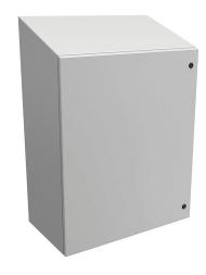
Hammond Eclipse series enclosure, slope top, NEMA 3R/4/12,  $36 \times 30 \times 16$  in (HxWxD), wall mount, carbon steel, RAL 7035 light gray, powder coat finish, single-door, 1/4-turn semi-flush latch.
