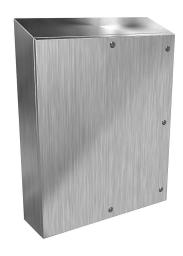
Hammond Eclipse series enclosure, slope top, NEMA 3R/4/4X/12/13,  $36 \times 30 \times 8$  in (HxWxD), wall mount, 304 stainless steel, #4 brush finish, single-door, 1/4-turn semi-flush 316 stainless steel latch.
