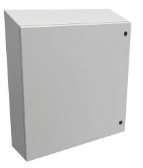
Hammond Eclipse series enclosure, slope top, NEMA 3R/4/12,  $30 \times 30 \times 8in$  (HxWxD), wall mount, carbon steel, RAL 7035 light gray, powder coat finish, single-door, 1/4-turn semi-flush latch.
