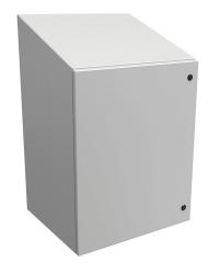
Hammond Eclipse series enclosure, slope top, NEMA 3R/4/12,  $30 \times 24 \times 20$  in (HxWxD), wall mount, carbon steel, RAL 7035 light gray, powder coat finish, single-door, 1/4-turn semi-flush latch.
