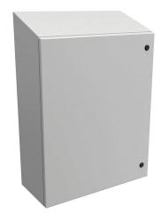
Hammond Eclipse series enclosure, slope top, NEMA 3R/4/12,  $30 \times 24 \times 10$  in (HxWxD), wall mount, carbon steel, RAL 7035 light gray, powder coat finish, single-door, 1/4-turn semi-flush latch.
