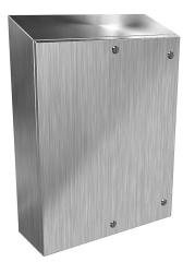
Hammond Eclipse series enclosure, slope top, NEMA 3R/4/4X/12/13,  $30 \times 24 \times 8in$  (HxWxD), wall mount, 304 stainless steel, #4 brush finish, single-door, 1/4-turn semi-flush 316 stainless steel latch.
