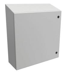
Hammond Eclipse series enclosure, slope top, NEMA 3R/4/12,  $24 \times 24 \times 8$  in (HxWxD), wall mount, carbon steel, RAL 7035 light gray, powder coat finish, single-door, 1/4-turn semi-flush latch.
