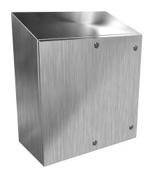
Hammond Eclipse series enclosure, slope top, NEMA 3R/4/4X/12/13, 24 x 24 x 12in (HxWxD), wall mount, 304 stainless steel, #4 brush finish, single-door, 1/4-turn semi-flush 316 stainless steel latch.
