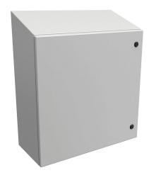
Hammond Eclipse series enclosure, slope top, NEMA 3R/4/12, 24 x 24 x 10in (HxWxD), wall mount, carbon steel, RAL 7035 light gray, powder coat finish, single-door, 1/4-turn semi-flush latch.
