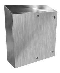
Hammond Eclipse series enclosure, slope top, NEMA 3R/4/4X/12/13,  $24 \times 24 \times 8$  in (HxWxD), wall mount, 304 stainless steel, #4 brush finish, single-door, 1/4-turn semi-flush 316 stainless steel latch.
