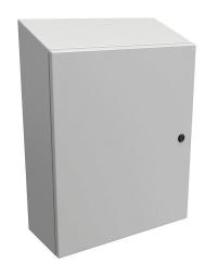
Hammond Eclipse series enclosure, slope top, NEMA 3R/4/12,  $24 \times 20 \times 8$  in (HxWxD), wall mount, carbon steel, RAL 7035 light gray, powder coat finish, single-door, 1/4-turn semi-flush latch.
