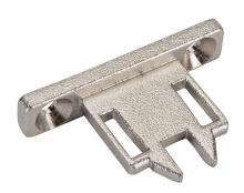
Dold Safemaster series, actuator tongue (key), 90 degree mounting tab mount, 316 stainless steel. For use with trapped key interlock systems.
