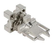
Dold Safemaster series, actuator tongue (key), shock absorbing, 90 degree mounting tab mount, 316L stainless steel. For use with trapped key interlock systems.
