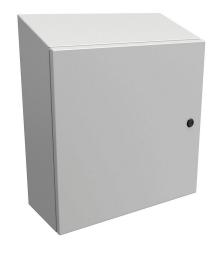
Hammond Eclipse series enclosure, slope top, NEMA 3R/4/12,  $20 \times 20 \times 8$ in (HxWxD), wall mount, carbon steel, RAL 7035 light gray, powder coat finish, single-door, 1/4-turn semi-flush latch.
