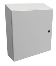
Hammond Eclipse series enclosure, slope top, NEMA 3R/4/12,  $20 \times 20 \times 6$  in (HxWxD), wall mount, carbon steel, RAL 7035 light gray, powder coat finish, single-door, 1/4-turn semi-flush latch.
