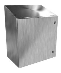
Hammond Eclipse series enclosure, slope top, NEMA 3R/4/4X/12/13,  $20 \times 20 \times 12$  in (HxWxD), wall mount, 304 stainless steel, #4 brush finish, single-door, 1/4-turn semi-flush 316 stainless steel latch.
