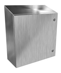
Hammond Eclipse series enclosure, slope top, NEMA 3R/4/4X/12/13,  $20 \times 20 \times 8$  in (HxWxD), wall mount, 304 stainless steel, #4 brush finish, single-door, 1/4-turn semi-flush 316 stainless steel latch.
