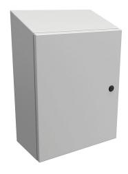
Hammond Eclipse series enclosure, slope top, NEMA 3R/4/12,  $20 \times 16 \times 8$  in (HxWxD), wall mount, carbon steel, RAL 7035 light gray, powder coat finish, single-door, 1/4-turn semi-flush latch.
