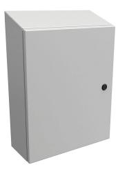
Hammond Eclipse series enclosure, slope top, NEMA 3R/4/12, 20 x 16 x 6in (HxWxD), wall mount, carbon steel, RAL 7035 light gray, powder coat finish, single-door, 1/4-turn semi-flush latch.
