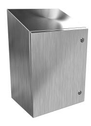
Hammond Eclipse series enclosure, slope top, NEMA 3R/4/4X/12/13,  $20 \times 16 \times 12$  in (HxWxD), wall mount, 304 stainless steel, #4 brush finish, single-door, 1/4-turn semi-flush 316 stainless steel latch.
