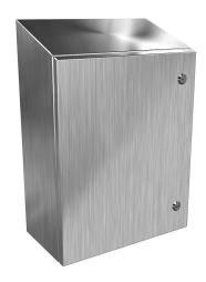
Hammond Eclipse series enclosure, slope top, NEMA 3R/4/4X/12/13,  $20 \times 16 \times 8$  in (HxWxD), wall mount, 304 stainless steel, #4 brush finish, single-door, 1/4-turn semi-flush 316 stainless steel latch.
