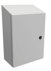
Hammond Eclipse series enclosure, slope top, NEMA 3R/4/12, 16 x 12 x 6in (HxWxD), wall mount, carbon steel, RAL 7035 light gray, powder coat finish, single-door, 1/4-turn semi-flush latch.
