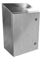
Hammond Eclipse series enclosure, slope top, NEMA 3R/4/4X/12/13,  $16 \times 12 \times 8in$  (HxWxD), wall mount, 304 stainless steel, #4 brush finish, single-door, 1/4-turn semi-flush 316 stainless steel latch.
