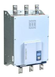
WEG Electric SSW900 series full-featured soft starter, 950A, 220-575 VAC at 3-phase, Trip Class 10/20/30, rated for 5 start/ hour, internally bypassed, F frame. Optional communication and RTD cards available.
