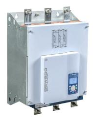
WEG Electric SSW900 series full-featured soft starter, 670A, 220-575 VAC at 3-phase, Trip Class 10/20/30, rated for 5 start/hour, internally bypassed, E frame. Optional communication and RTD cards available.
