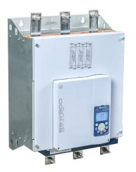
WEG Electric SSW900 series full-featured soft starter, 604A, 220-575 VAC at 3-phase, Trip Class 10/20/30, rated for 5 start/ hour, internally bypassed, E frame. Optional communication and RTD cards available.
