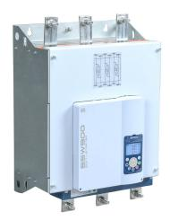
WEG Electric SSW900 series full-featured soft starter, 480A, 220-575 VAC at 3-phase, Trip Class 10/20/30, rated for 5 start/hour, internally bypassed, E frame. Optional communication and RTD cards available.
