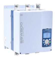
WEG Electric SSW900 series full-featured soft starter, 412A, 220-575 VAC at 3-phase, Trip Class 10/20/30, rated for 10 start/hour, internally bypassed, D frame. Optional communication and RTD cards available.
