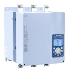
WEG Electric SSW900 series full-featured soft starter, 312A, 220-575 VAC at 3-phase, Trip Class 10/20/30, rated for 10 start/hour, internally bypassed, D frame. Optional communication and RTD cards available.
