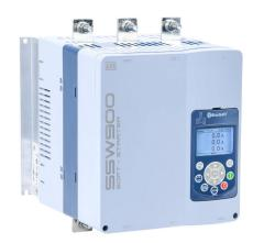
WEG Electric SSW900 series full-featured soft starter, 200A, 220-575 VAC at 3-phase, Trip Class 10/20/30, rated for 3 start/hour, internally bypassed, C frame. Optional SSW0708900-KVT-3C fan provides 10 start/hour. Optional communication and RTD cards available.
