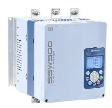
WEG Electric SSW900 series full-featured soft starter, 171A, 220-575 VAC at 3-phase, Trip Class 10/20/30, rated for 3 start/hour, internally bypassed, C frame. Optional SSW0708900-KVT-3C fan provides 10 start/hour. Optional communication and RTD cards available.
