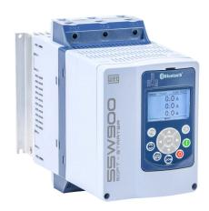
WEG Electric SSW900 series full-featured soft starter, 105A, 220-575 VAC at 3-phase, Trip Class 10/20/30, rated for 3 start/hour, internally bypassed, B frame. Optional SSW0708900-KVT-2B fan provides 10 start/hour. Optional communication and RTD cards available.
