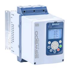
WEG Electric SSW900 series full-featured soft starter, 61A, 220-575 VAC at 3-phase, Trip Class 10/20/30, rated for 3 start/hour, internally bypassed, B frame. Optional SSW0708900-KVT-2B fan provides 10 start/hour. Optional communication and RTD cards available.
