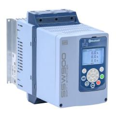
WEG Electric SSW900 series full-featured soft starter, 45A, 220-575 VAC at 3-phase, Trip Class 10/20/30, rated for 3 start/ hour, internally bypassed, B frame. Optional SSW0708900-KVT-2B fan provides 10 start/hour. Optional communication and RTD cards available.
