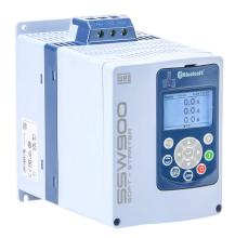
WEG Electric SSW900 series full-featured soft starter, 17A, 220-575 VAC at 3-phase, Trip Class 10/20/30, rated for 10 start/hour, internally bypassed, A frame. Optional communication and RTD cards available.
