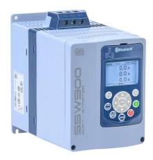
WEG Electric SSW900 series full-featured soft starter, 10A, 220-575 VAC at 3-phase, Trip Class 10/20/30, rated for 10 start/hour, internally bypassed, A frame. Optional communication and RTD cards available.
