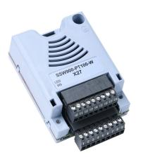
WEG Electric SSW900 series temperature input module, RTD, 6-channel, 12-bit resolution, input RTD type(s): Pt100. For use with WEG SSW900 series soft starters. Removable terminal block included.
