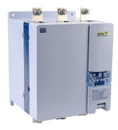
WEG Electric SSW07 series basic soft starter, 412A, 220/460/575 VAC at 3-phase, Trip Class 5/10/20/30, rated for 10 start/hour, internally bypassed. Optional Modbus RTU cards available.
