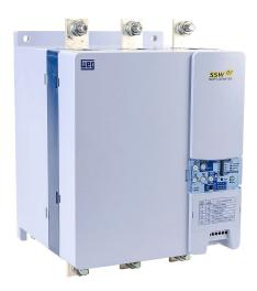
WEG Electric SSW07 series basic soft starter, 312A, 220/460/575 VAC at 3-phase, Trip Class 5/10/20/30, rated for 10 start/hour, internally bypassed. Optional Modbus RTU cards available.
