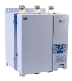
WEG Electric SSW07 series basic soft starter, 255A, 220/460/575 VAC at 3-phase, Trip Class 5/10/20/30, rated for 10 start/hour, internally bypassed. Optional Modbus RTU cards available.
